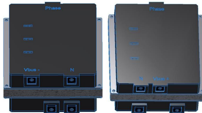
Fig. III-45. Lower (left) and upper (right) power modules placed on the evaporator
