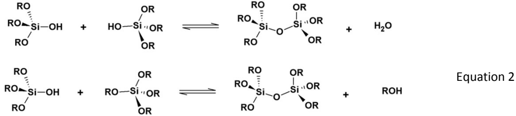
Scheme S1. Hydrolysis and condensation reactions of the sol-gel process.
