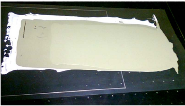
Fig. 9. Tape obtained by sequential tape casting, showing electrolyte, functional, and structural anode layers.
