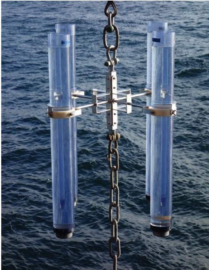
Fig 3.6: The four gyroscopically mounted sediment trap collection tubes.
