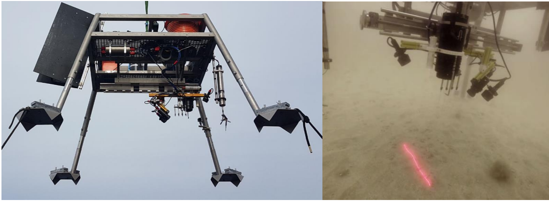
Fig. 3.10: Left panel: LanceALot after a 24 hour deployment on the Mauretania shelf. Right panel: Surface-scan of the sea-floor using a laser-scanning technique.
