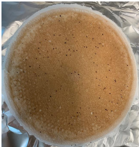
Fig 3.3: POC filter with plenty of particulate material. 50 L of seawater from the ship inlet were filtered using a peristaltic pump through 0.47 µm GF/F filters with a diameter of 142 mm.
