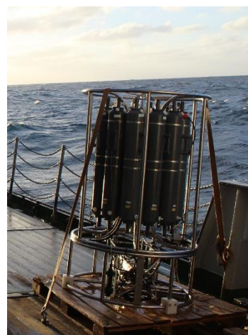
Fig. 3.4: CTD rosette ready for deployment.
