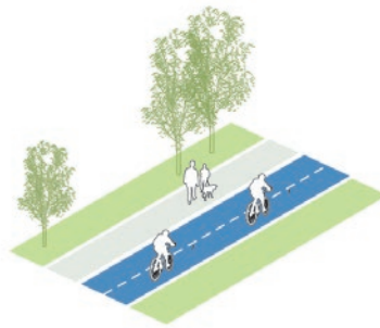
separated bicycle and pedestrian paths in limited spaces enhanced by material, colour and level difference
