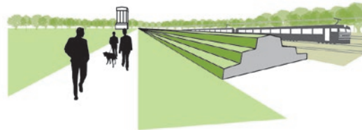
Image 83, My example of an earth berm with stepped profile that could mitigate noise in Kroņu Street, Riga. Image designed and drafted by myself and based on principles from HOSANNA project ( HOSANNA Summary Brochure, 2013 )
