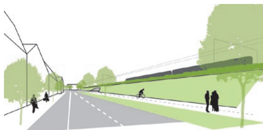
Image 85, My example of a low weight vegetated barriers at the bridges that could mitigate noise in Satekles Street, Riga. Image designed and drafted by myself and based on principles from HOSANNA project ( HOSANNA Summary Brochure, 2013 )
