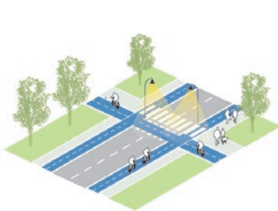
safe bicycle and pedestrian street crossings enhanced by colour and street lights
