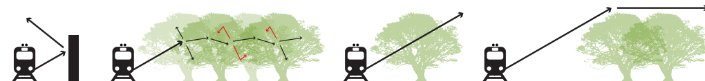
The image 77. Processes of noise distribution, Illustration is designed and drafted by myself and based on information from Environmental Methods for Transport Noise Reduction (Nilsson, M. E. , Bengtsson, J. , Klæboe, R. 2015, p.79)
