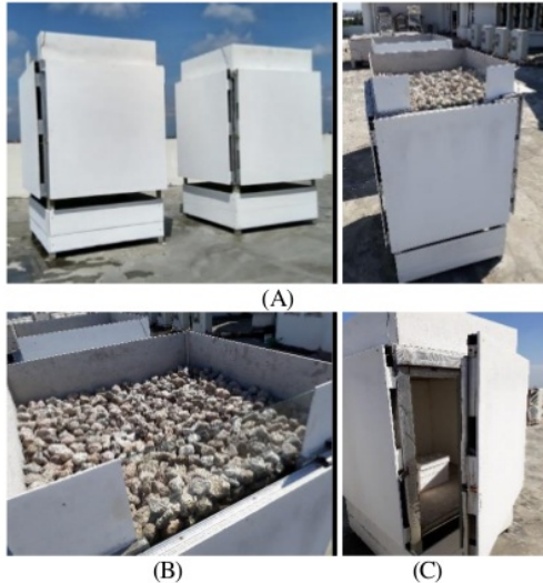
Fig. 7. Two Experimental Models (A), Pumice Rooftop (One model) (B), Measured Room Model (C)
