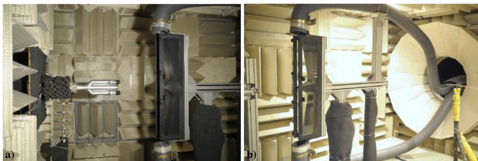
Fig. 6 View of a) the model inside the anechoic chamber, and b) the pipes taking out exhaust from the deflector.
