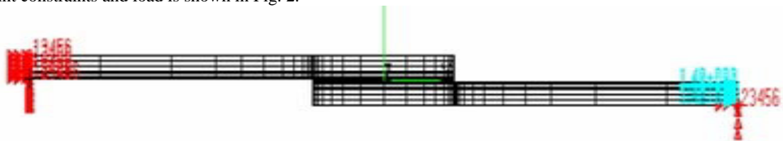
Fig.2. 2-D FE model with boundary conditions, MPC and load
