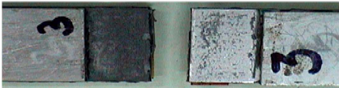
Fig.5. Failure surface of CFRP-Al adhesively bonded joint
