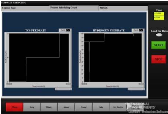
Fig. 7. Characteristics of TCS and Hydrogen feedrate as scheduled
