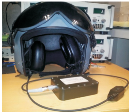
Fig. 2. The ANC Unit Integrated with the Fighter Aircraft Pilot Helmet.
