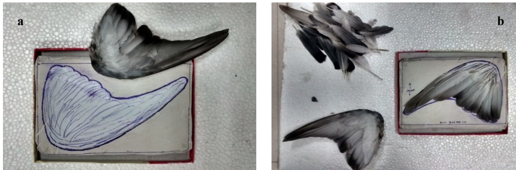
Fig. 8. (a) developed mold using natural pigeon wing; (b) artificial wing preparation using feathers.
