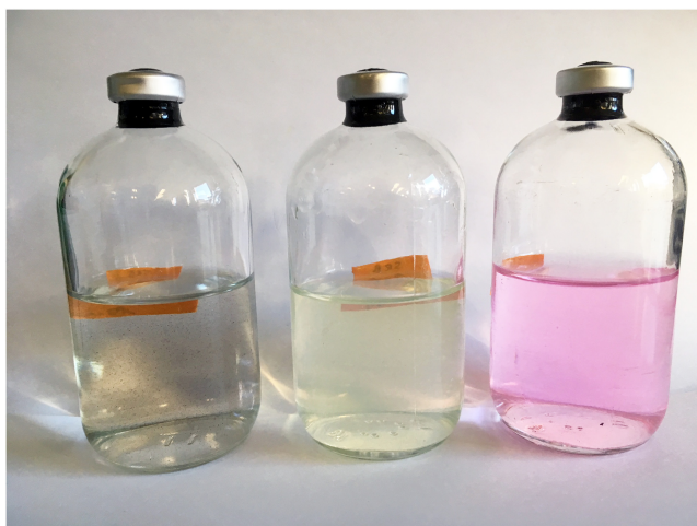
Figure 4 | The culture medium in serum bottles. (Left) Medium prepared under strictly anoxic conditions appears colorless with small black precipitates. (Middle) Yellowish medium indicates formation of elemental sulfur in the culture medium due to minor oxygen contamination. (Right) Medium has turned pink due to an increase of redox potential by contamination with more oxygen.
