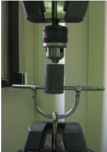
Fig. 1 Specimen in customized self-aligning testing assembly mounted in universal testing machine.
