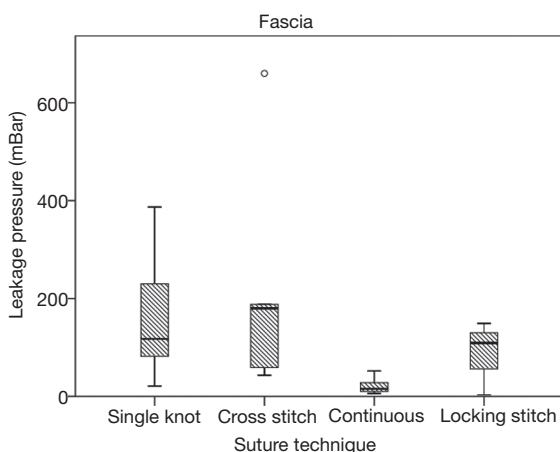
Figure 6 For fascia closure, cross stitch (median =180 mbar) resulted in a significantly higher leakage pressure than continuous (median =16 mbar) ( P=0.003 ) but not than single knot (median =118 mbar) ( P=1.0 ) and locking stitch suture (median =109 mbar) ( P=0.93 ).
