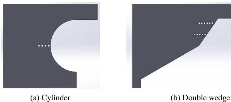
Figure 2.13: SolidWorks drawings of alignment plates used for position calibration.
