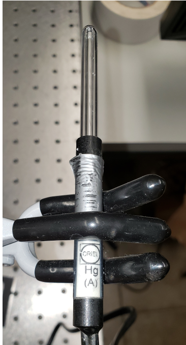
Figure 2.19: Mercury-argon lamp mounted for instrument line shape measurement.
