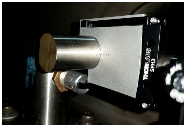
Figure 2.14: Alignment of spatial calibration plate over the surface of a cylinder model inside the HET test section.
