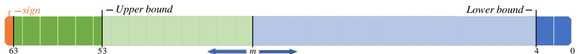
Figure 5: Visualization of the length limits of the mantissa on a 64-bit long backend
