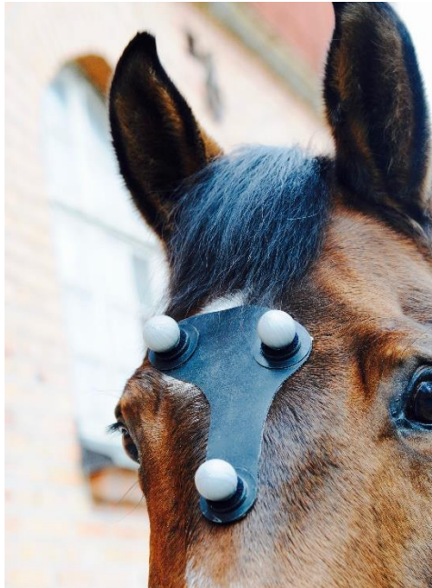
Figure 3. Frontal plane spherical reflective markers used on some horses in Paper IV, the ventral midline marker was used in the analysis (Photo: Elin Holmroos).
