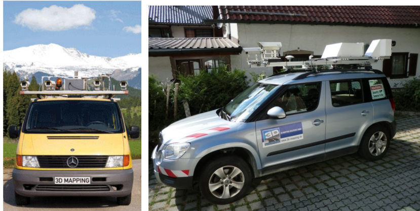
Figure 10: Mapping vehicles used for the initial creation of the HD Map used during the Ko-HAF Project. ©3D Mapping Solutions GmbH.
