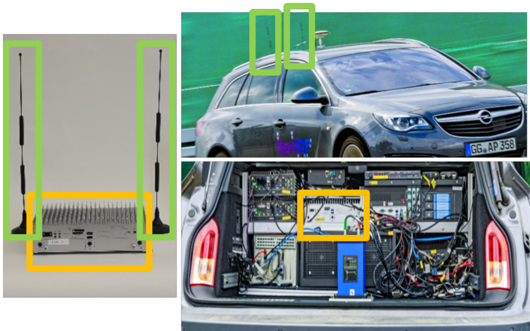
Figure 73: The common communication box installed in all twelve vehicles, that participated in the Ko-HAF Project. The box provided communication functionalities via all cellular network technologies (4G, 3G and 2G), that were deployed during the duration of the Ko-HAF project (September 2015 - November 2018). ©Ko-HAF, Opel Automobile GmbH 39
