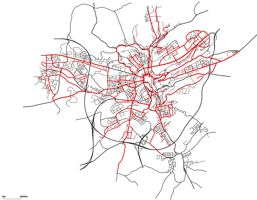
Figure 91: Visualisation of the LUST dataset [109] of the area of Luxembourg for the traffic simulator SUMO. The streets where buses are roaming in the map are indicated by red color. (Source: https://github.com/lcodeca/LuSTScenario/blob/master/docs/img/LuST_busCoverage.png (Last accessed on August 1, 2019))
