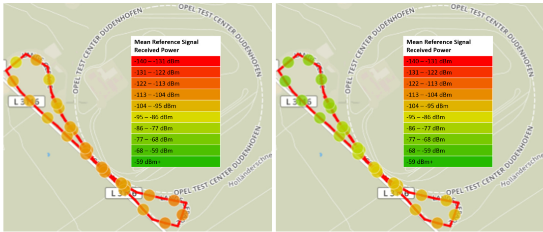
(a) Measured Reference Signal Received Power at the first day of the measuring campaign on the site (07.11.17).
