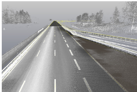
(c) Visualisation of Laser Scanner data used for HD Map generation - ©3D Mapping Solutions GmbH
