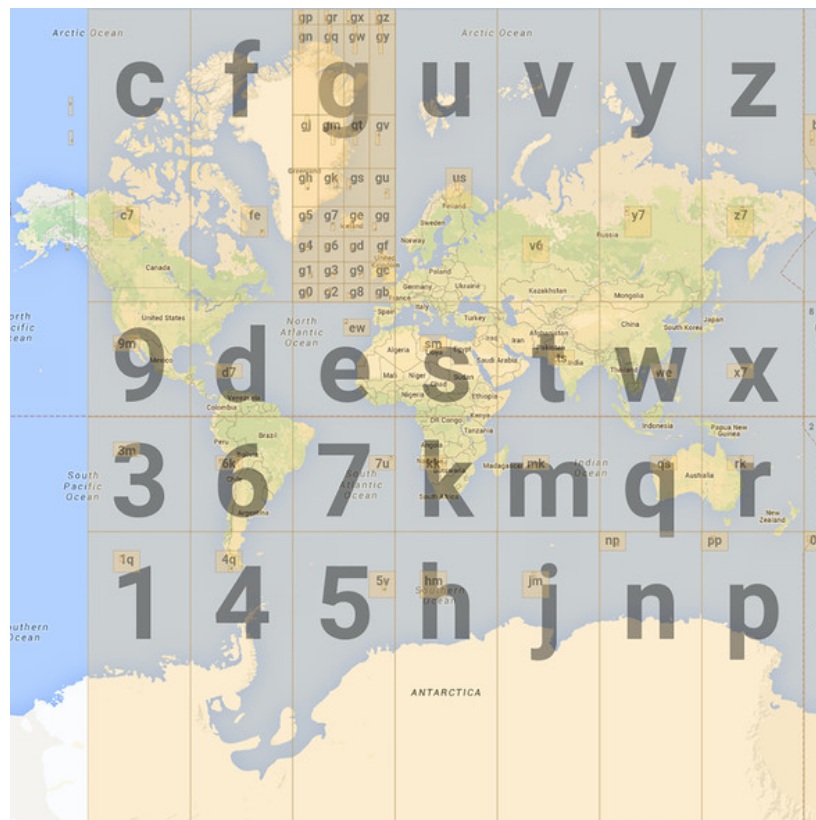
Figure 7: Example visualization of nearby Geohashes of different accuracy levels. The higher accuracy is indicated by longer strings. Neighbouring strings start with the same sequence of letters. (Source: https://www.movable-type.co.uk/scripts/geohash.jpg (Last accessed on August 1, 2019))
