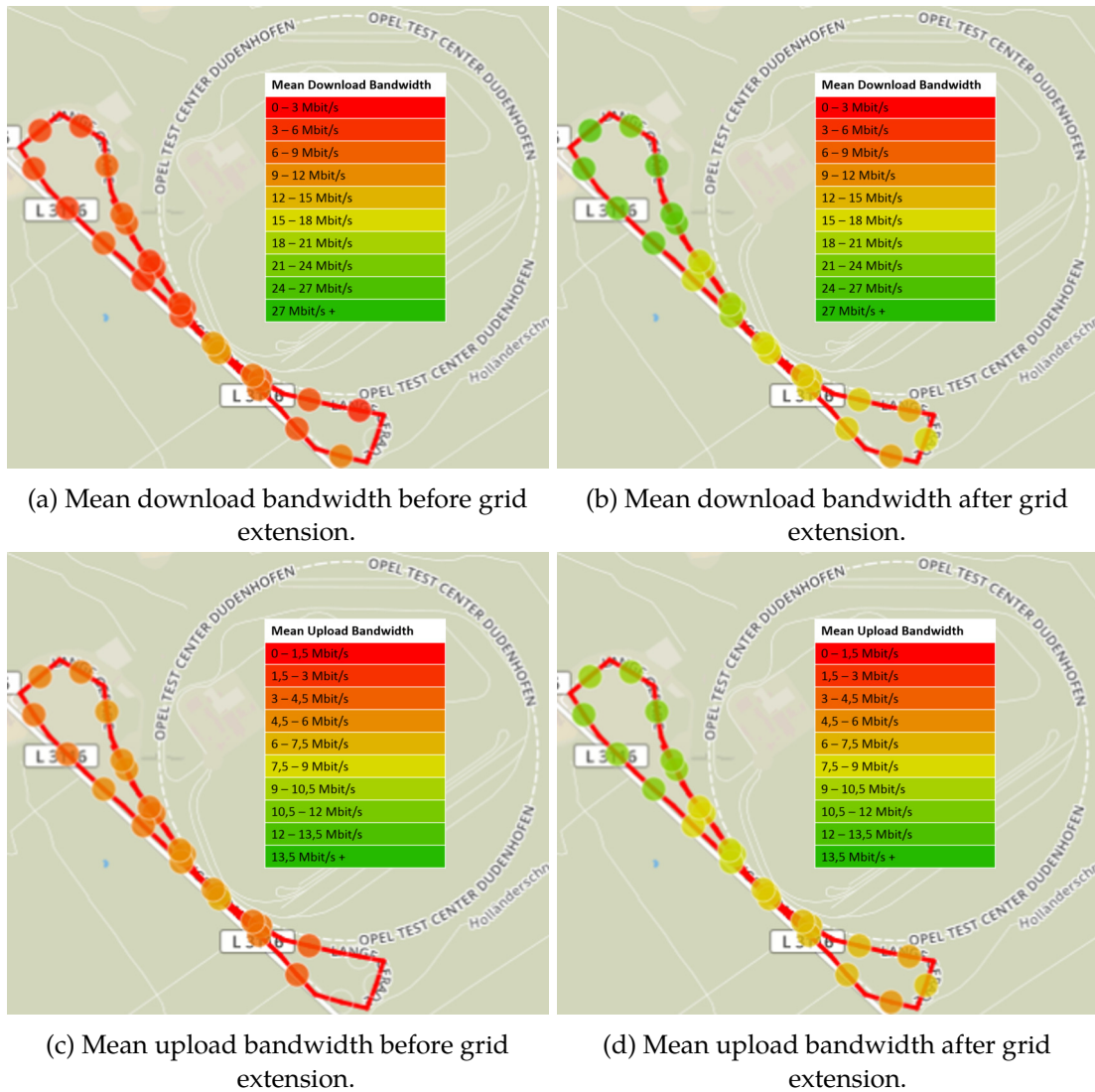
Figure 84: Comparison of mean average download and upload bandwidth of the provider Vodafone as measured at the Opel proving ground in Rodgau Dudenhofen before (07.11.2017-29.01.2018) and after (29.01.2018-20.09.2018) the LTE grid extension. Map data ©OpenStreetMap contributors
