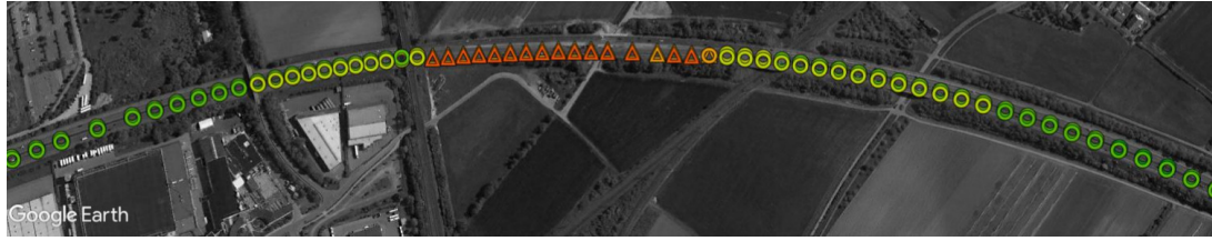
Figure 34: Correlation between the average vehicles speed (indicated by color) and the location of the construction site (indicated by triangles). Speeds right before and in the construction site range from 90 km/h down to 57 km/h (yellow - red). Before and after the construction site normal driving speeds of around 125 km/h are reached in average (green) [89]. Satellite image ©Google Earth
