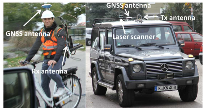
Fig. 5: Antennas positions on both the test vehicle and the cyclist.
