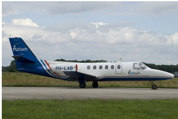
Fig. 5 Cessna Model 550 Citation II Research Aircraft PH-LAB [25].
