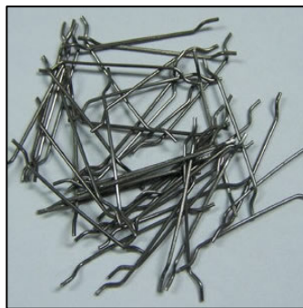
Figure 2: Hooked End Steel Fibre
