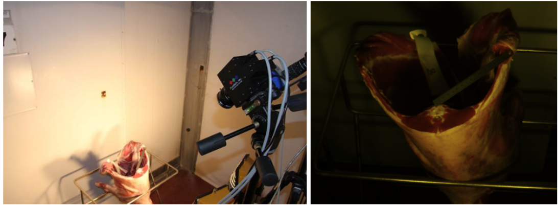
Figure 2.2: Hyperspectral imaging acquisition stage. Left panel shows the setup of the Hyperspectral equipment. Right panel shows the recovered pseudo-colour image of a sheep carcass. Adapted from Robles-Kelly and R. Wei (2015)
