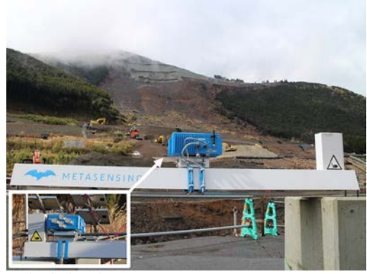
Fig. 1. The deployed GB-SAR system.
