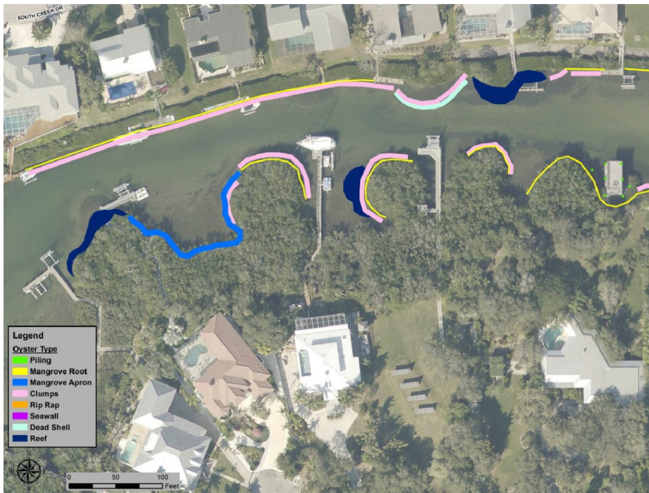
Figure 5.5. Example of the detail of oyster mapping completed in Sarasota Bay. Image credit: Meaux et al. 2016.
