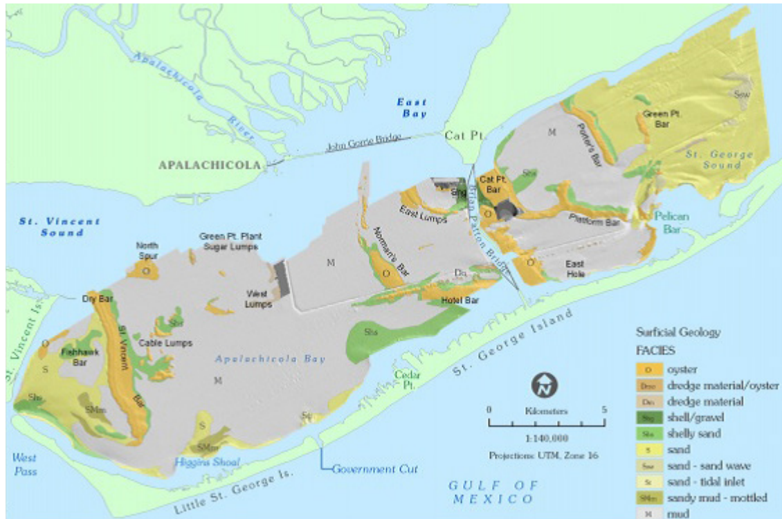
Figure 3.9. Composite map of the surficial geology of Apalachicola Bay based on 2005–2006 sonar-based mapping. (Figure from Twichell et al. 2007.)
