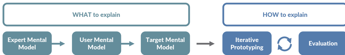
Figure 3.3: Our stage-based participatory design process for designing user support in real-world settings. The first three stages focus on what to explain in the system (information), the last two on how to explain (presentation).
