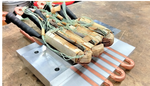
Fig. 6. Cold plate assembly before clamping: motorette, interface plate and water-glycol cooled 6-pass cold plate.
