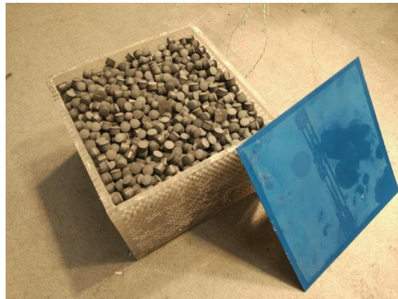
Figure 5: Filled box with activated alumina before fins insertion and plate fixation.
