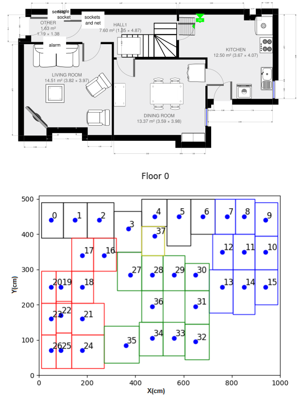
Figure 3. Example of discretised floor plan, for the use with fingerprinting. Figure above shows the corresponding floor plan. Below, each discretised state is 1 meter apart. Different colours of the grids signify different rooms. These approaches have been proven to be notoriously arduous in labour, especially in large industrial and commercial spaces. Image courtesy of Byrne et al. [13]
