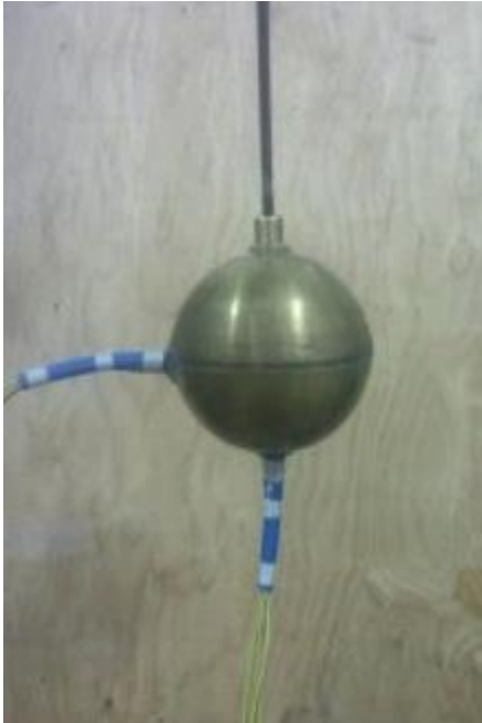
Figure 4: Test section after applying thermocouples
