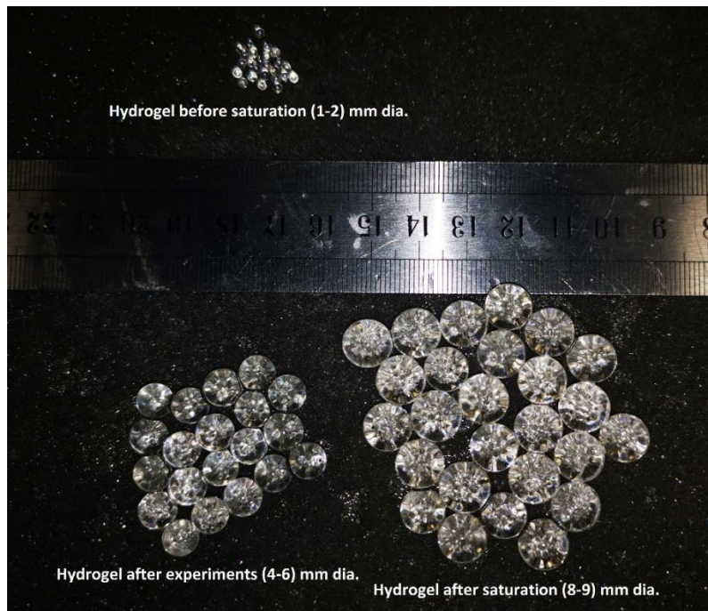
Figure 5: Hydrogel spheres before saturation, after saturation and after experiments.
