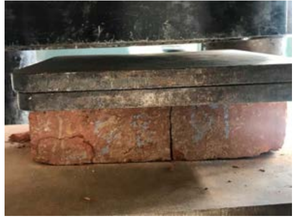
Figure 3. Experimental setup for compressive tests of fired bricks carried out at the Tribhuvan University (SAFER, 2019b).
