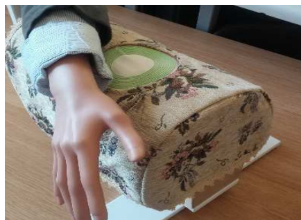
Figure 1. An Illustrative mock-up of the IPT system for powering wrist worn sensors
