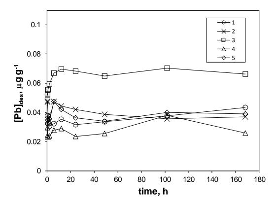
Figure 2: Concentration of Pb adsorbed to five pellet types (defined in Table 1) that is released by an
