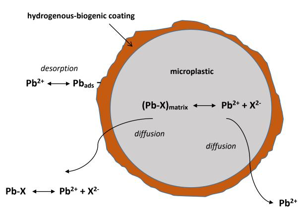
Figure 1: Associations of Pb (and other metals) with microplastics in the marine environment and mechanisms by which they are released. Note that Pb-X represents an additive or residue in the polymeric matrix.
