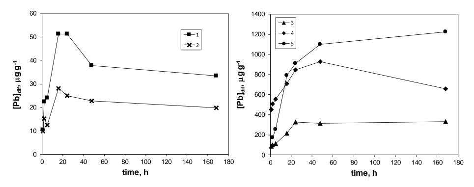
Figure 3: Concentration of Pb as an additive in five micronized plastics (defined in Table 1) that is released by an avian PBET, [Pb]<sub>dif</sub>, as a function of time.
