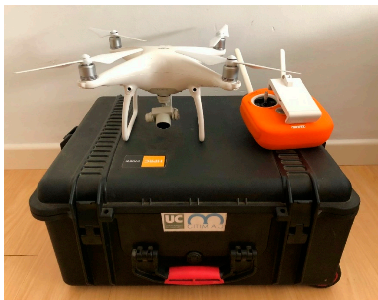
Figure 4. Quadricopter DJI Phantom 4 employed for surveying the mining remains.
