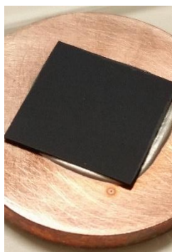
Fig. 31: Assembling of the mold compound sample onto a copper electrode via a heat conducting glue.
