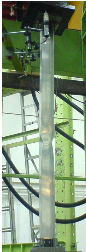
(b) Specimen P-T6-L1350 (failure mode: local and flexural buckling)
