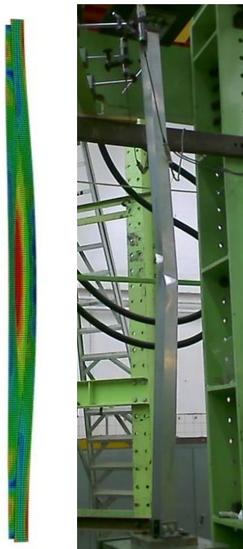
(d) Specimen P-T6-L2450 (failure mode: local, flexural and flexural-torsional buckling)
