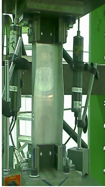
(a) Specimen P-T5-L300 (failure mode: local buckling)
