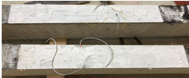
(e) Finished surface after 28 days of curing
