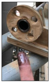
Figure 5: Oil traces found in the secondary leakage line.
