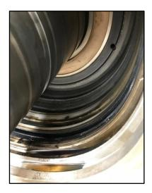
Figure 9: Dry gas seal found with oil contamination leakage during replacement.
