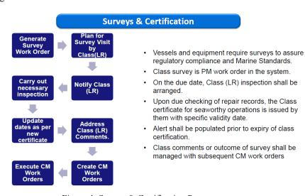
Figure 4: Survey & Certification Process
