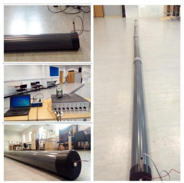
**Figure 2** – The experimental set-up, sensor attached, pc and DAC, loudspeaker etc
