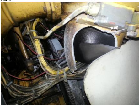
Figure 1: Elbow (7.5"), 8mm thickness Exploded
