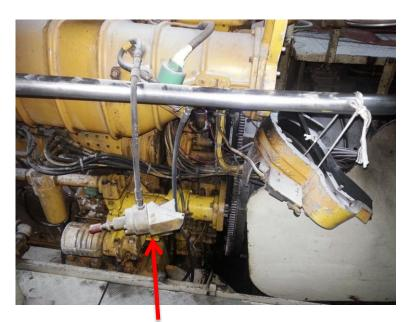
Emergency Shut off Device (Expecting Flap Operated)
