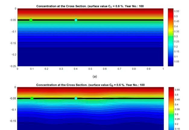
**Figure 2.** Distribution of chloride concentration in homogeneous model (**a**) at the age of 100 years, including the scheme of the conventional reinforcement (black line) and random field based model (**b**) at the age of 100 years including the scheme of the epoxy-coated reinforcement (black line) and locations of the holidays in the reinforcement epoxy coating (Epo<sub>1</sub> = green circle, Epo<sub>2</sub> = blue rhombus).
