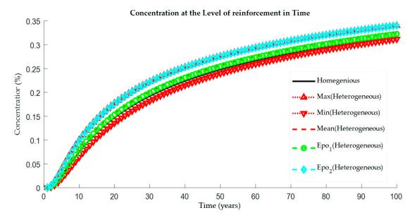
**Figure 3.** Increase of chloride concentration over the time at reinforcement level for the homogeneous and random field based model for the deterministic solution. The homogeneous model represents both conventional steel reinforcement as well as an epoxy-coated. While the heterogeneous denoted Max, Min and Mean represent the conventional steel. The Epo<sub>1,2</sub> refer to an epoxy-coated heterogeneous model.
