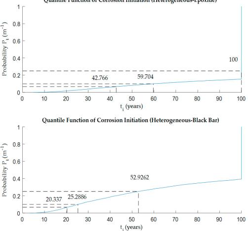
**Figure 5.** Probability of corrosion initiation,  $t_i$ , from the heterogeneous model—black bar vs. epoxy-coated reinforcement.
