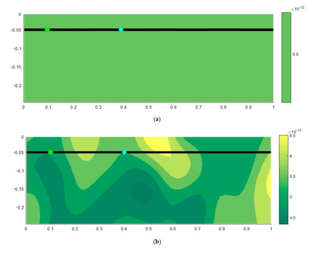
**Figure 1.** Distribution of the diffusion coefficient in homogeneous model (**a**) including the scheme of the conventional reinforcement (black line) and random field based model (**b**) including the scheme of the epoxy-coated reinforcement (black line) and locations of the holidays in the reinforcement epoxy coating (Epo<sub>1</sub> = green circle, Epo<sub>2</sub> = blue rhombus).
