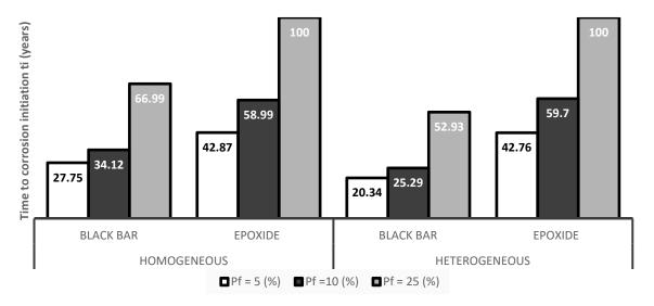
**Figure 6.** Period to the initiation of corrosion,  $t_i$  (years), for a selected probability level for studied models.
