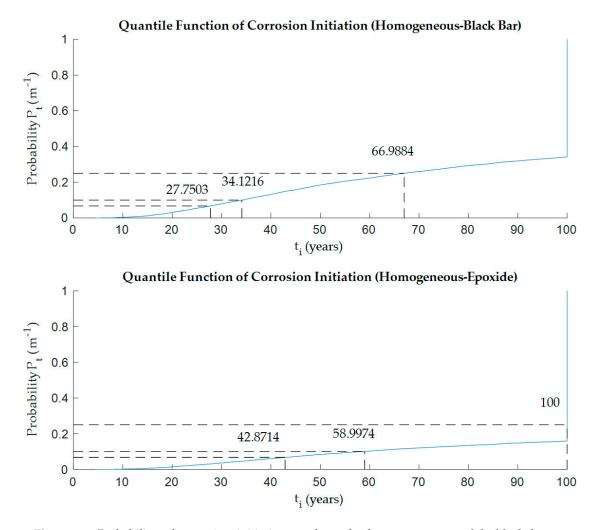
**Figure 4.** Probability of corrosion initiation,  $t_i$ , from the homogeneous model—black bar vs. epoxy-coated reinforcement.
