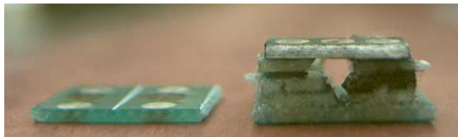
Figure 11 Self-assembly substrate and final substrate after completion of self-assembly process.
