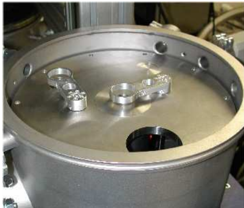
Figure 2: Multiple rakes and powder supplies allow varying compositions
