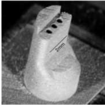
Fig 7a: Grip bit for the positioning of an optical lens
