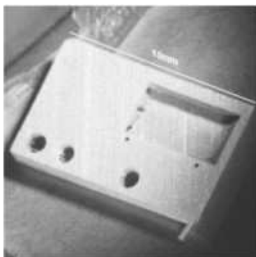
Fig 9a: Aspiration box of the fiber holder
