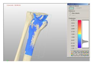
Figure 6: Error map of the physical model for the case of a distal tibia
