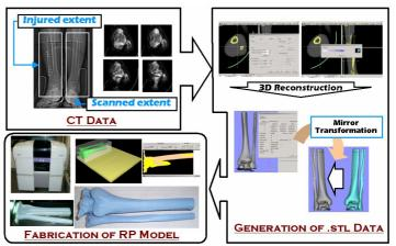
Figure 5: Procedure from CT data to the fabrication of rapid prototyping model of a distal
