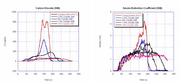
**Figure 6 and 7** Comparison of carbon monoxide yield (left) and smoke extinction coefficient (right) for 2.5, 5, 7.5, 10 wt% of Cloisite® 30B PA11N at 50 kW/m<sup>2</sup> heat flux.
