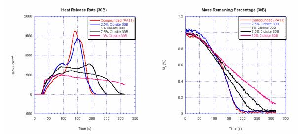
**Figures 4 and 5** Comparison of heat release rate (left) and residue mass (right) for 2.5, 5, 7.5, 10 wt% of Cloisite® 30B PA11N at 50 kW/m<sup>2</sup> heat flux.
