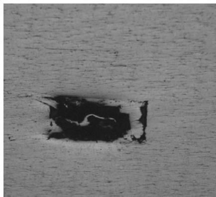
Fig.14. Free-standing ribs built at a 45° orientation. Exposed gaps between adjacent strips of tape.
