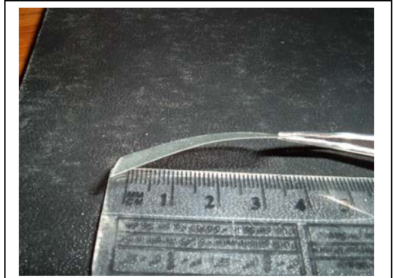
Figure 5: Neat HDODA printed film 30 layers, 140 \mu\text{m} thick
