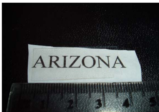
Figure 3: Neat HDODA printed film 140 \mu m thick, 30 layers; the film is flexible
