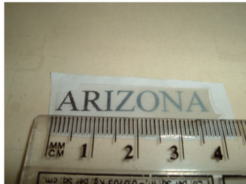
Figure 4: Gradient printed film containing 0 to 4.5wt% SiC; 140 \mu m thick, 30 layers
