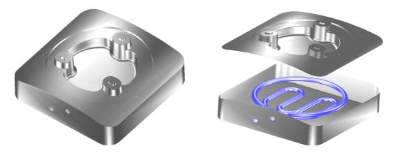
Figure 2: Left: injection molding tool insert, right: view of the internal cooling system
