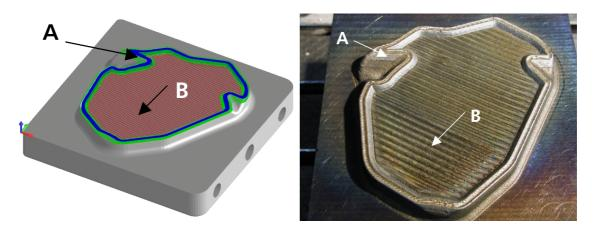
Figure 7: Generation of tools using laser-/ plasma build-up welding
