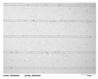
Figure 3: Cross-section of a brazed tool
