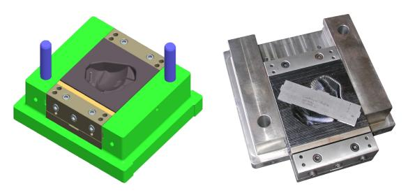
Figure 6: Universal tool frame concept for a stamping die
