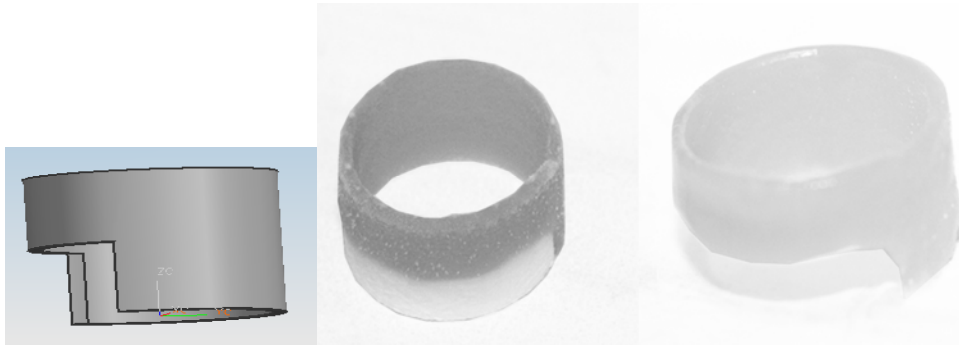
Figure 15: A cylinder built in -23^{\circ}\text{C} ambient, a) concept, b) before and c) after support material removal
