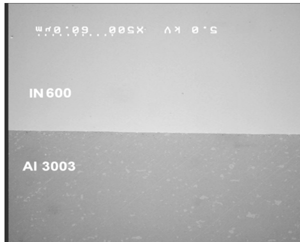
Fig.6. SEM microstructure of directly welded Al 3003/IN 600.
