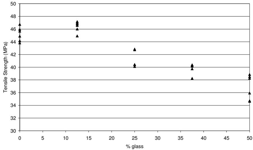
Figure 3 - Tensile Strength
