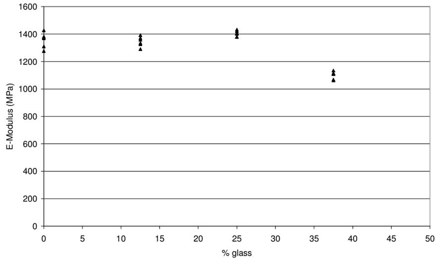
**Figure 5 - Flexural Modulus**
