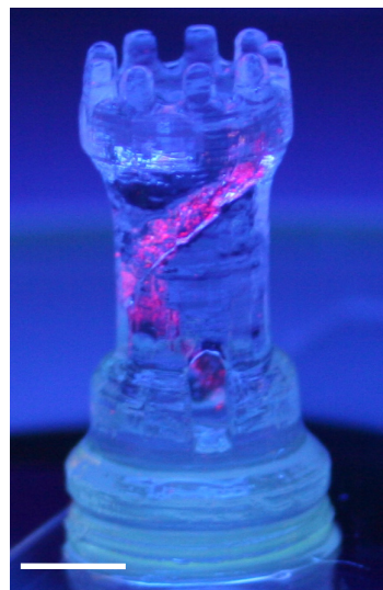
Figure 7. Complex 3D structure manufactured in multi-material SL. PEG-dma 1K at a 20% (w/v) concentration was used as the main material. The solution used to create the staircase contained fluorescent microspheres. Scale bar represents 5mm.
